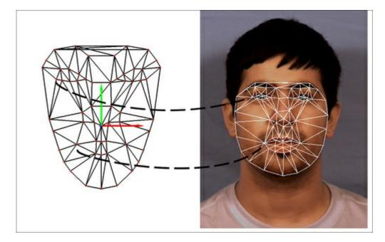
The preceding screenshot shows the correctly matched points of a 3D head model and an AAM mesh.
