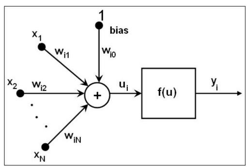
There are three widely used activation functions: Identity, Sigmoid, and Gaussian; the most common and default activation function is the Sigmoid function. It has an alpha and beta value set to 1:
