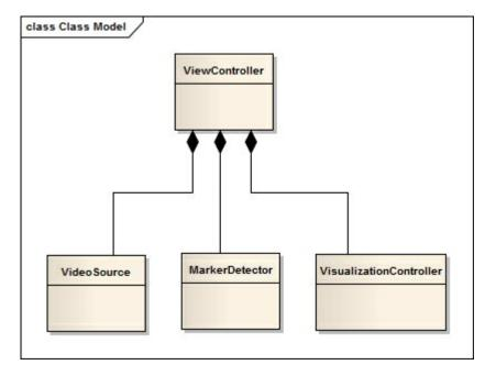
The video source is responsible for providing new frames taken from the built-in camera to the user code. This means that the video source should be capable of choosing a camera device (front- or back-facing camera), adjusting its parameters (such as resolution of the captured video, white balance, and shutter speed), and grabbing frames without freezing the main UI.
