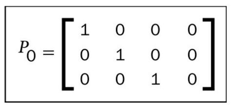
The other camera that we recovered from the essential matrix has moved and rotated in relation to the fixed one. This also means that any of the 3D points that we recover from these two camera matrices will have the first camera at the world origin point (0, 0, 0).
