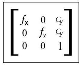
We're mainly interested in four components: fx, fy, cx, and cy. With this data we can create an instance of the camera-calibration object using the following code for calibration:
