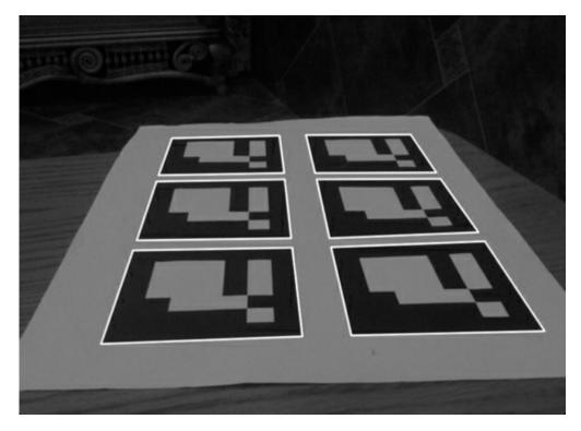
We do not use cornerSubPix in the earlier stages of marker detection due to its complexity. It's very expensive to call this function for large numbers of points (in terms of computation time). Therefore we do this only for valid markers.
