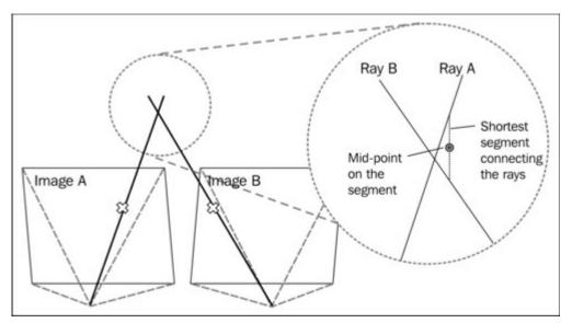
In reality, ray intersection is highly unreliable; H and Z recommend against it. This is because the rays usually do not intersect, making us fall back to using the middle point on the shortest segment connecting the two rays. Instead, H and Z suggest a number of ways to triangulate 3D points, of which we will discuss a couple of them in the Reconstructing the scene section. The current version of OpenCV does not contain a simple API for triangulation, so this part we will code on our own.
