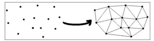
This screenshot is the output of the preceding code for a set of points that yield the triangulation using Delaunay algorithm.
