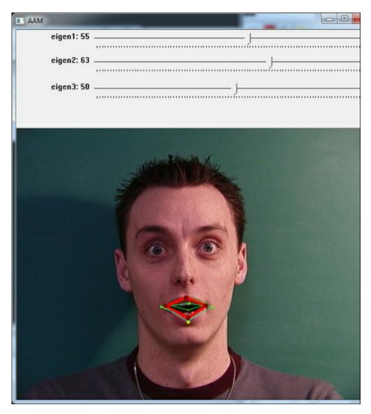
The two previous screenshots show two different shape configurations according to the selected parameters chosen from the slider. The yellow and green shapes show training data, while the red one reflects the shape generated from the chosen parameters.
