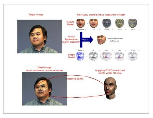
Overview of the chapter algorithms: Given an image (upper-left image in the preceding screenshot), we can use an Active Appearance search algorithm to find the 2D pose of the human head. The upper-right side figure in the screenshot shows a previously trained Active Appearance model used in the search algorithm. After a pose has been found, POSIT can be applied to extend the result to a 3D pose. If the procedure is applied to a video sequence, 3D tracking by detection will be obtained.
