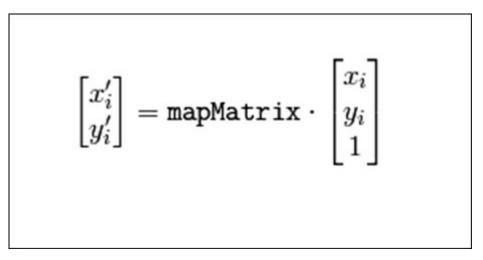
In the preceding equation, destination (i) is equal to (xi',yi'), source (i) is equal to (xi, yi), and i is equal to 0, 1, 2.
