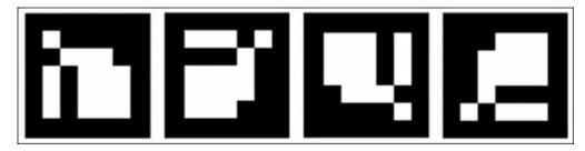
As there are four possible orientations of the marker picture, we have to find the correct marker position. Remember, we introduced three parity bits for each two bits of information. With their help we can find the hamming distance for each possible marker orientation. The correct marker position will have zero hamming distance error, while the other rotations won't.
