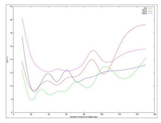
We can see that the lowest error is under 8 percent and is using 20 neurons in a hidden layer and characters' features extracted from a downscaled  $10 \ge 10$  image patch.
