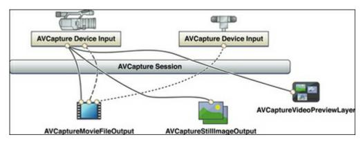
AVCaptureSession is a root capture object that we should create. Capture session requires two components—an input and an output. The input device can either be a physical device (camera) or a video file (not shown in diagram). In our case it's a built-in camera (front or back). The output device can be presented by one of the following interfaces:
