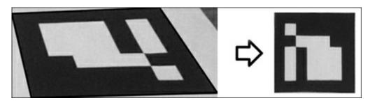
Now we can test the image to verify if it is a valid marker image. Then we try to extract the bit mask with the marker code. As we expect our marker to contain only black and white colors, we can perform Otsu thresholding to remove gray pixels and leave only black and white pixels:
